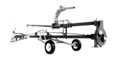
**BOTTOM AGITATION GUNS -** this model is especially effective for use in lagoons with heavy bottom solids, which are common in swine operations. The gun is located near the bottom of the lagoon so that the agitation stream can be directed at the bottom solids to break them up and homogenize them into the lagoon slurry. This allows the lagoon to be managed more effectively and eliminates diminishing lagoon capacity due to bottom sludge build-up.
