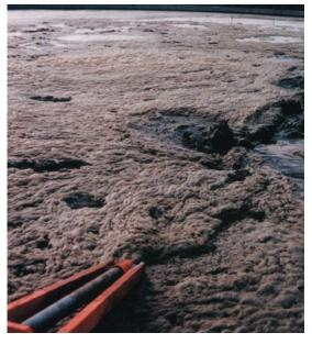
The 130' diameter pit, 12' deep, was dairy and hog waste. A 23" diameter propeller running at 1000 RPM agitated this pit from one location.
